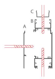
**3.** Attach the mounting strip (A) to the mounting surface with screws suitable for the mounting surface. Run the cable out through the gland.
