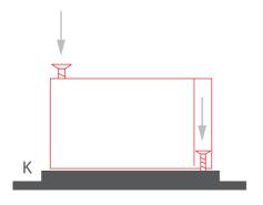
**2.** Insert the cable gland (O) and the spacers (N) into the holes in the mounting strip (A).
