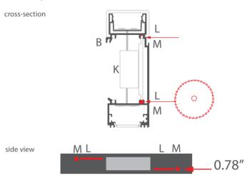
**8.** Connect power and assemble the extrusion (B) with the mounting strip (A).
